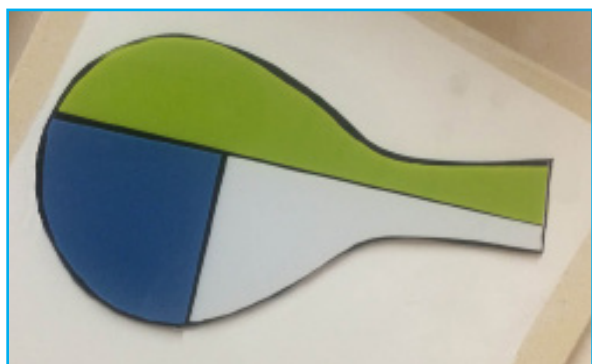
The base glass with design layer on kiln shelf paper ready to fuse.
